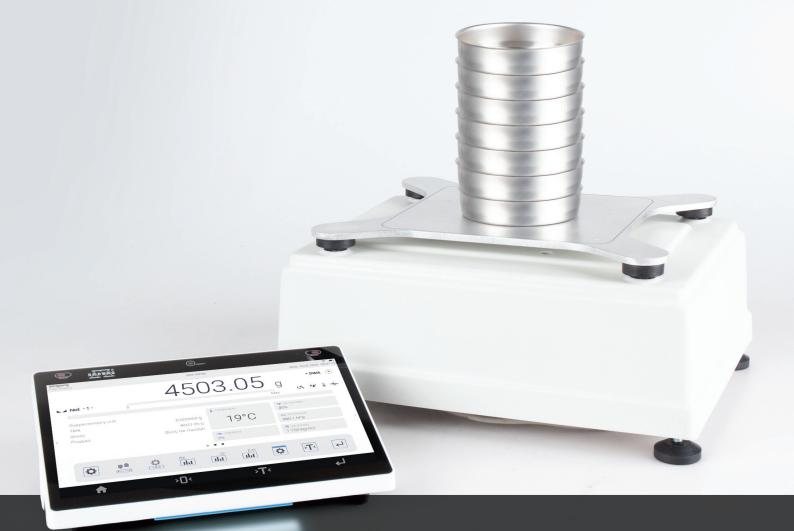
The PM 20.5Y laboratory balance by Radwag is one of the most innovative in the world that can weigh up to 20 kg with 0.01 g readability, using a large 200 x 185 mm weighing pan.
