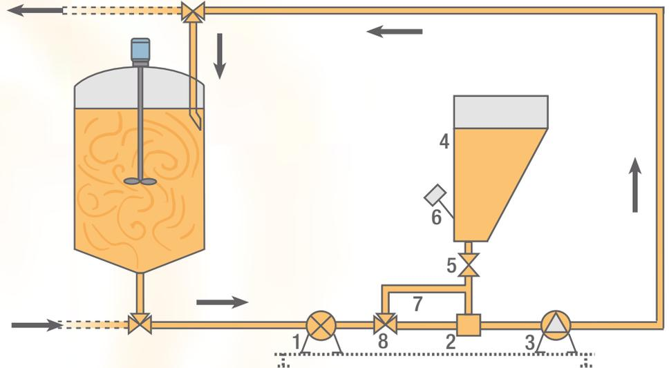
the valve, minimising aeration. When the powder sensor closes the powder feed valve, product flow can be diverted round a bypass line (7) by the diverter valve (8).
