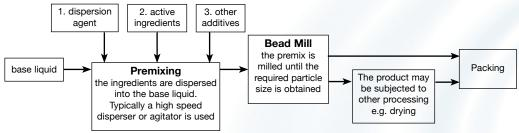
Processing with a media mill such as a bead mill
